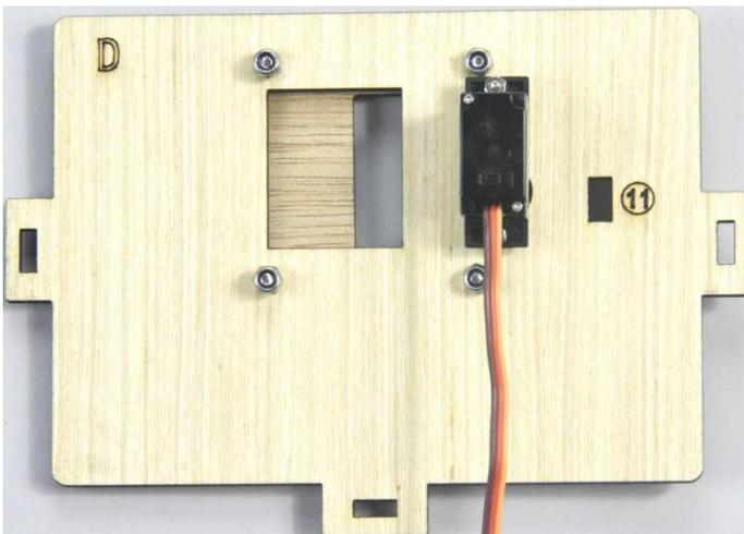
Step 6: Assemble C board with D board by a "T" type bolt.
